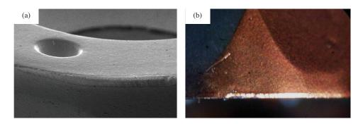
FIGURE 3. Typical tool wear mode during machining Inconel 718 (a) SEM image of chipping, abrasion, adhesion and attrition on cutting edge and rake surface (b) microscope view
