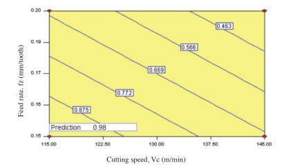
FIGURE 8. Contour plot of the statistically recommended parameters to obtain the longest predicted tool life within the parameter limit, where  $a_a = 0.50$  and  $a_a = 0.15$
