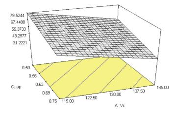
FIGURE 5. Interaction effect between axial depth of cut and cutting speed
