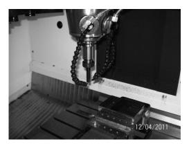
FIGURE 1. Position of MQL nozzles in the high speed milling
