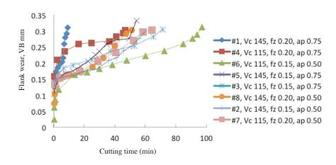
FIGURE 2. Flank wear development of PVD coated in milling Inconel 718, at various parameters
